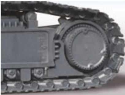
The O&K specific transmission of power avoids wear-intensive relative movement between track and sprocket.
