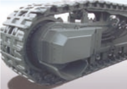
Encapsulated, powerful two-stage travel motors are the key for mobility. Easy access to components due to hinged doors.
